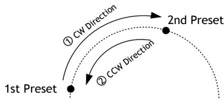
In case that the preset assigned as the 1st point is same as the preset assigned as the 2nd point, camera turns on its axis by 360° in CW(Clockwise) direction and then it turns on its axis by 360° in CCW(Counterclockwise) direction.
