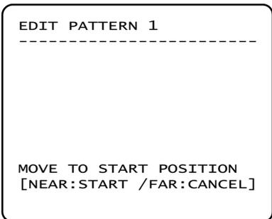
① By using Joystick, move to start position with appropriate zoom. To start pattern recording, press **NEAR** key. To exit this menu, press **FAR** key.
