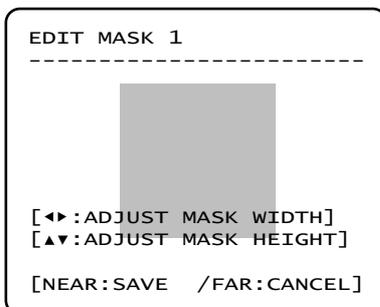
Adjust mask size. Use joystick or arrow buttons to adjust mask size.
