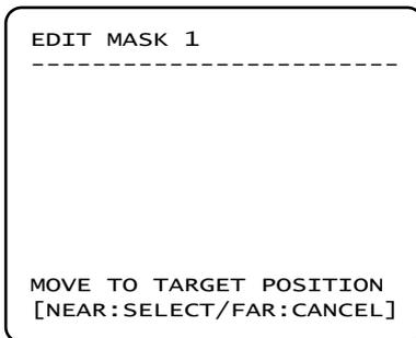
Move camera to area to mask. Then the menu to adjust mask size will be displayed.
