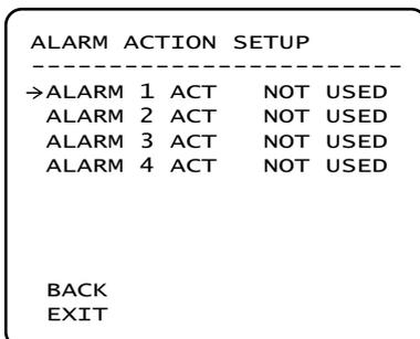
Match the Alarm sensor input to one of Preset positions. If an external sensor is activated, camera will move to corresponding preset position when this item is predefined.
