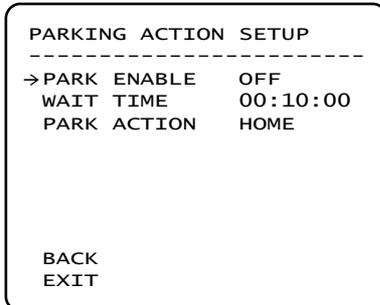
If Park Enable is set to ON, camera runs assigned function automatically if there is no PTZ command during assigned "Wait Time".
