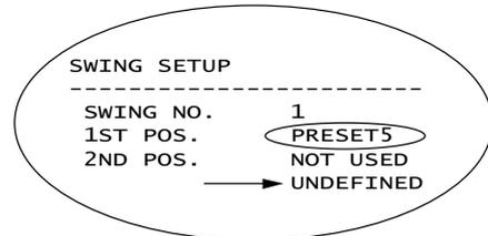
When swing function runs, camera moves from the preset assigned as the 1st point to the preset assigned as the 2nd point in CW(Clockwise) direction. Then camera moves from the preset assigned as the 2nd point to the preset assigned as the 1st point in CCW(Counterclockwise) direction. In case that the preset assigned as the 1st point is same as the preset assigned as the 2nd point, camera turns on its axis by 360° in CW direction and then it turns on its axis by 360° in CCW direction.
