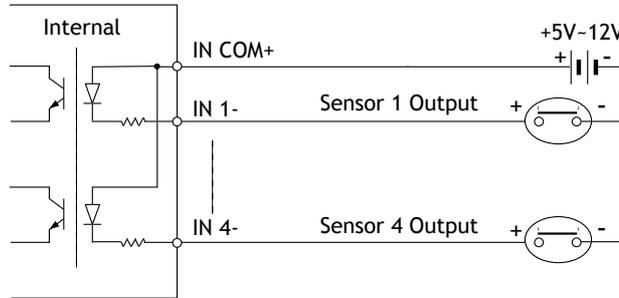
Before connecting sensors, check driving voltage and output signal type of the sensor. Since output signal types of the sensors are divided into Open Collector and Voltage Output type in general, the cabling must be done properly after considering these types. Also, the sensor type, i.e. “Normal Open” or “Normal Close” in Dip switch in main body of camera must be set properly.
