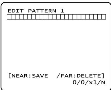
② Move camera with joystick of controller or run preset function to memorize the path (mostly curve path) in a selected pattern. The total memory size and the rest memory size is displayed in the form of bar. Maximum 1200 communication commands can be stored in a pattern.
