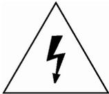
This lightning flash with arrowhead symbol is intended to alert the user to the presence of un-insulated "dangerous voltage" within the product's enclosure that may be of sufficient magnitude to constitute a risk of electric shock to persons.
