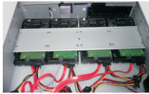
⑤ Install other three lower HDDs.
