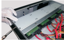
⑥ Install back the upper mounting bar.
