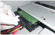
④ Connect the power and data cables.
