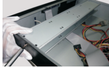
② Loosen the upper mounting bar.
