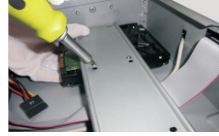
③ Screw HDD under the lower mounting bar.
