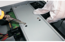
⑦ Screw HDD under upper mounting bar.
