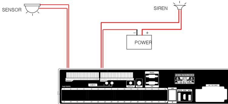
**Sensor In :** Connect the sensors. The sensor are composed of both signal and ground terminals, with a voltage difference of 5V. In the case that the sensor used for input is of the N/O (Normal Open) type, when the voltage difference between the signal and ground falls to 0V (short), the NVR can use this as a trigger to start alarm/sensor based recording.
