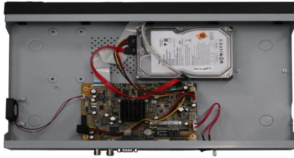
Figure 2. 8 Place the HDD on the bottom
