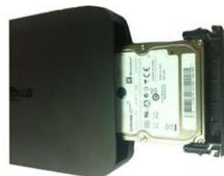
③ Put the HDD into the device
