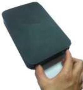
① Draw out the HDD bracket
