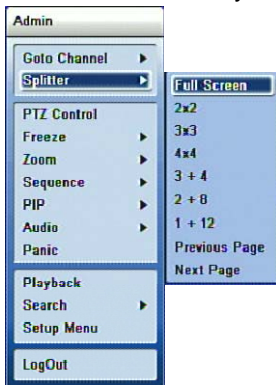
Figure 49 Splitter in Live view
